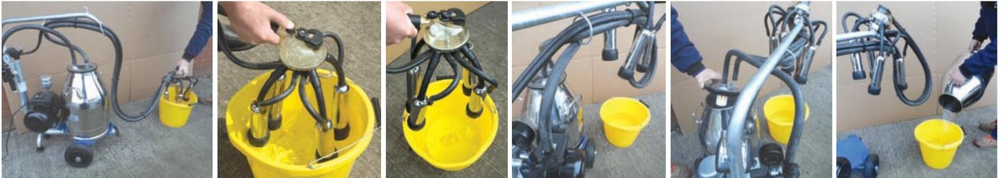
4. When the bucket is empty leave the pump running, turn off the vacuum tap to the bucket, remove the lid of the bucket and tip the water away.
