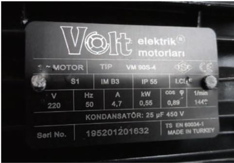
Figure 1: Label containing identification data of the electric motor.
